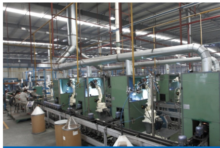
Shell Welding Line 壳体焊接
